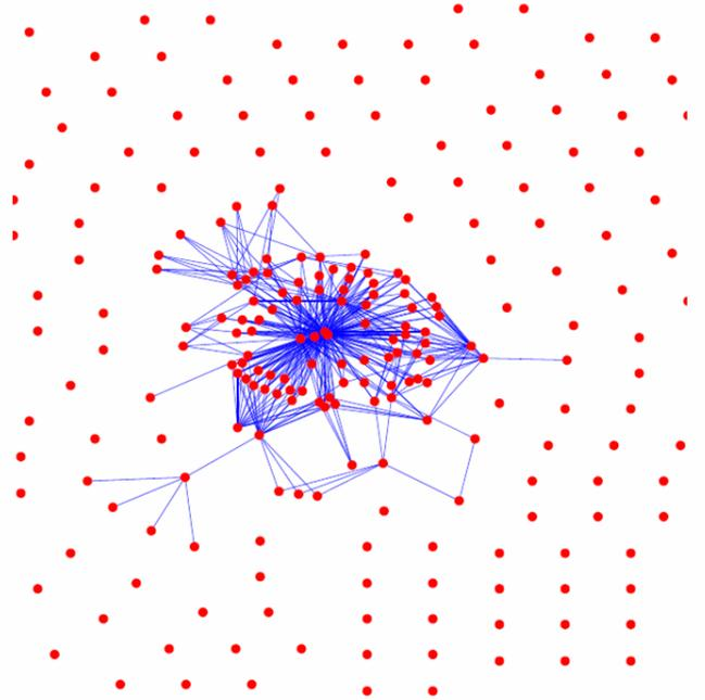
Figure 8: The IEEE 300-bus network has been redrawn here to highlight the structure of the electrical connections represented in the  $Z^{bus}$  matrix. To make this representation size-compatible with the topological representation in Figure 3, only the 411 strongest electrical connections (out of 44,700 total electrical connections) are shown.
