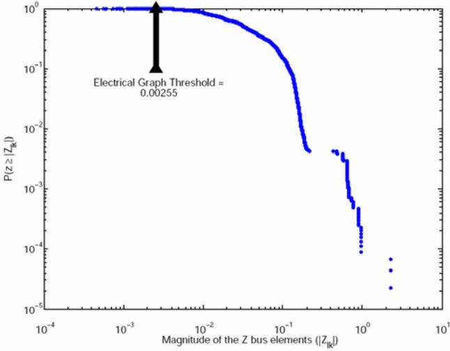
Figure 9: The inverse cumulative probability distribution function for all node-to-node electrical connections. The threshold at which only 411 stronger (smaller  $|Z_{ik}^{bus}|$ ) connections exist is 0.00255, as indicated.
