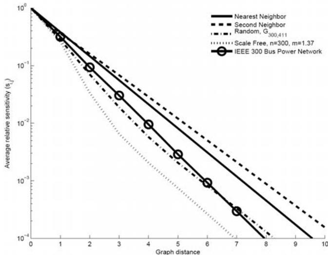
Figure 12: Average relative sensitivity  $S_{ij}$  plotted against the distance between  $i$  and  $j$ , for networks of resistors with different structures. For a given physical distance, the sensitivity is generally larger in the IEEE 300-bus network than in random or scale-free networks of approximately the same size. Information thus propagates more slowly in the 300-bus network than it would if the network had a scale-free or random structure.
