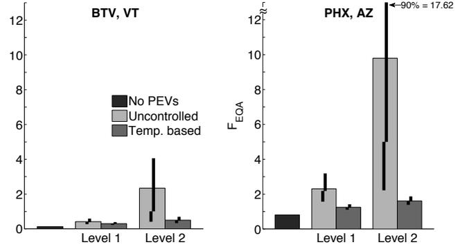
Figure 4. The annual factor of equivalent aging ( $F_{EQA}$ ) for Burlington, VT & Phoenix, AZ for no PEVs, uncontrolled PEV charging, and temperature-based smart charging. The graph displays average (bars) and 10<sup>th</sup> – 50<sup>th</sup> & 50<sup>th</sup> – 90<sup>th</sup> percentile (black lines)  $F_{EQA}$  values for each location and charging rate.
