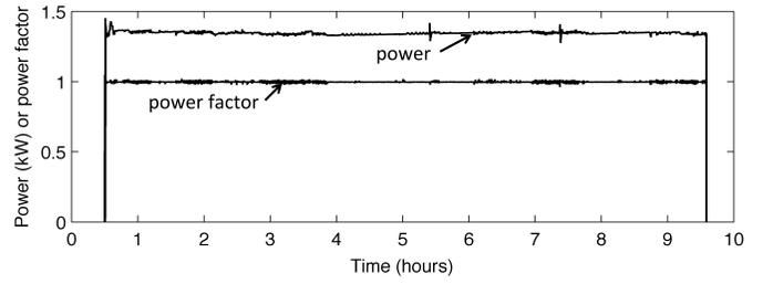
Figure 2. AC power consumption and power factor for a full (AC Level 1) charge of a GM Volt. Data courtesy of Central Vermont Public Service.
