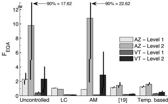
Figure 5. Transformer aging ( $F_{EQA}$ ) results for uncontrolled charging, and four smart-charging methods: load cutting (LC), after midnight (AM), randomized charging [19], and our temperature-based method. The graph displays average (bars) and  $10^{th} - 50^{th}$  &  $50^{th} - 90^{th}$  percentile (black lines)  $F_{EQA}$  values for each location and charging rate.
